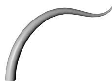
Branch Object with a Curvature Spline consisting of 20 Segments without Cubic Interpolation. The curve is slightly different than above, although the Spline parameters are the same.
